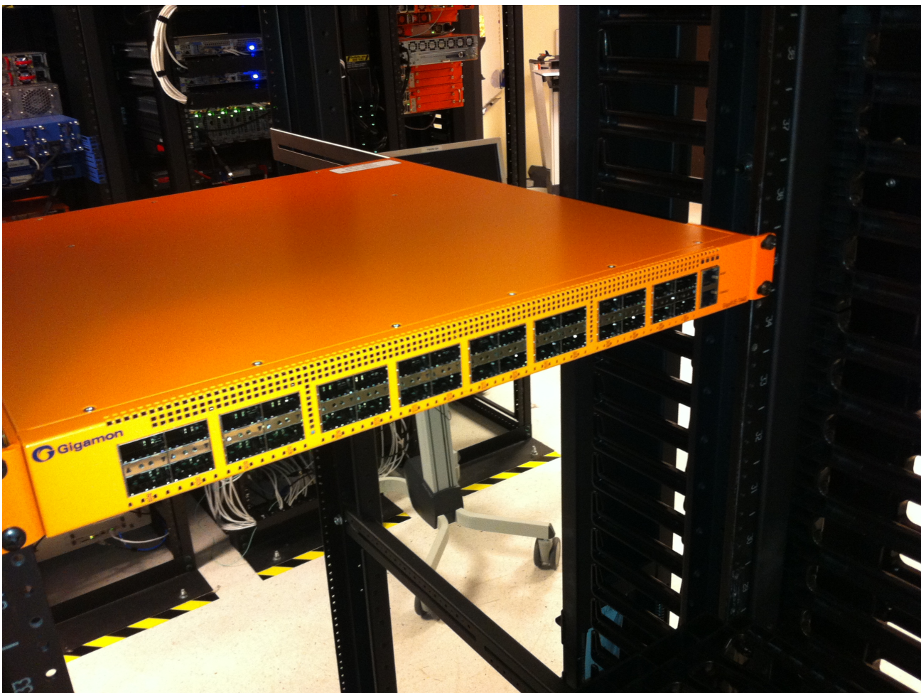
Figure 4 Front View of the Mounted Node to the Four-Post Rack
