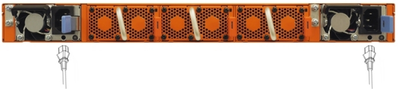
Figure 9 Connecting AC Power on a GigaVUE TA Series-TA100
